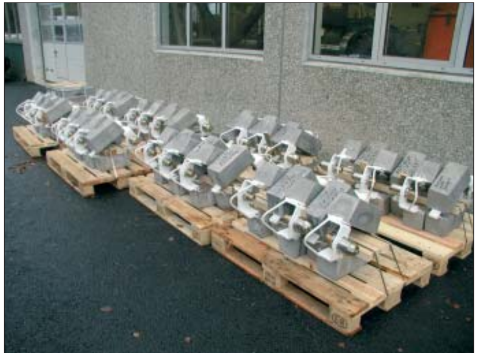
48 anodes completed and ready for shipment to Norsk Hydro. Anode #48 is produced as a spare anode with loose insert to fit the anchor line or the Pull In Tube support structure.
