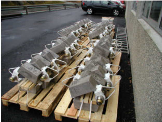
Anodes for installation on Troll B
