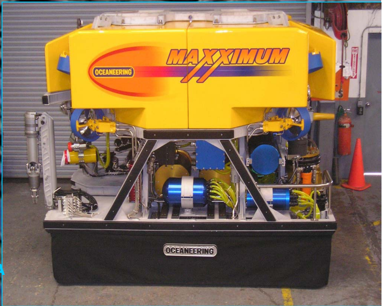
The 220SHP 'MAXXIMUM©' Construction ROV
