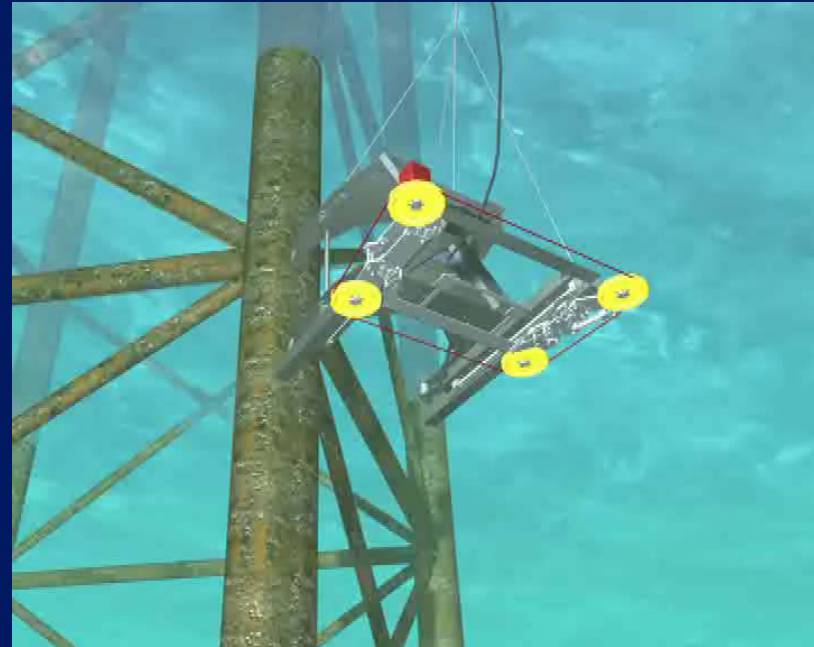
Diamond wire cutting (in figure above represented by Tecnoस्पamec DWC)
